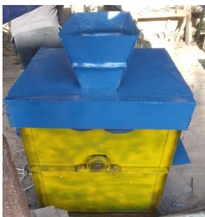
Figure 3. Improved cotton peeling machine from fine impurities of the new design
